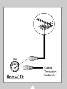
To view television channels correctly, a signal must be received by the set from one of the following sources:
